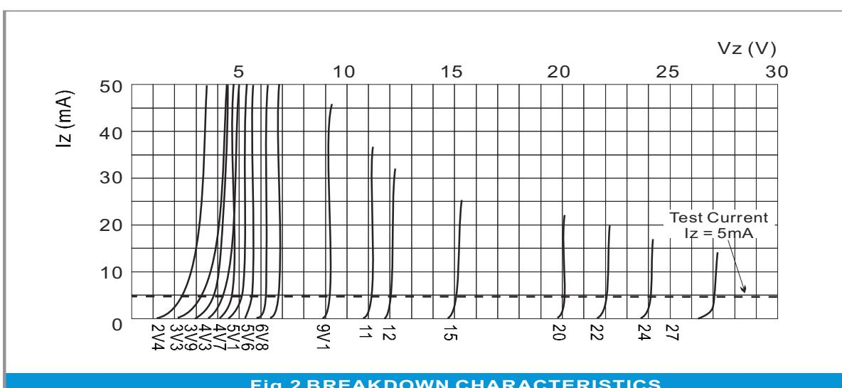
Fig.2 BREAKDOWN CHARACTERISTICS
