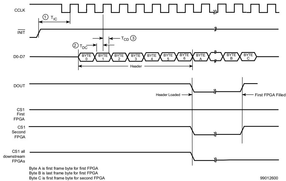
Note: CS1 must remain High throughout loading of the configuration data stream. In the pseudo daisy chain of Figure 5, the 7 byte data stream header is loaded into all devices simultaneously. Each device's data frames are then loaded in turn when its CS1 pin is driven High by the DOUT of the preceding device in the chain.
