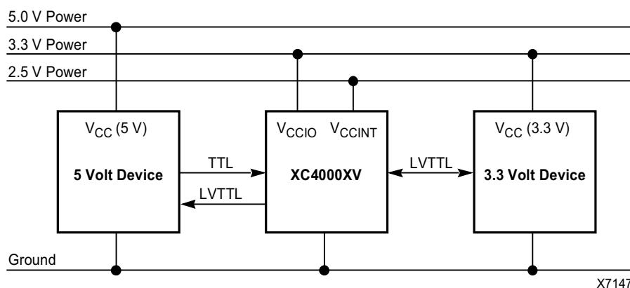
**Figure 4: The Signalling Environment for XLA/XV FPGAs.** For XLA devices the VCCIO and VCCINT supplies are replaced by a single 3.3 Volt VCC supply, however, all indicated I/O signalling is still supported.
