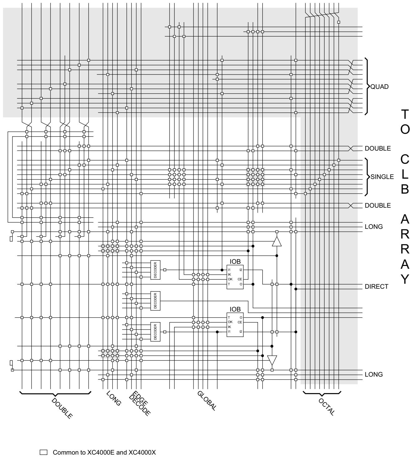
Figure 33: Detail of Programmable Interconnect Associated with XC4000 Series IOB (Left Edge)
