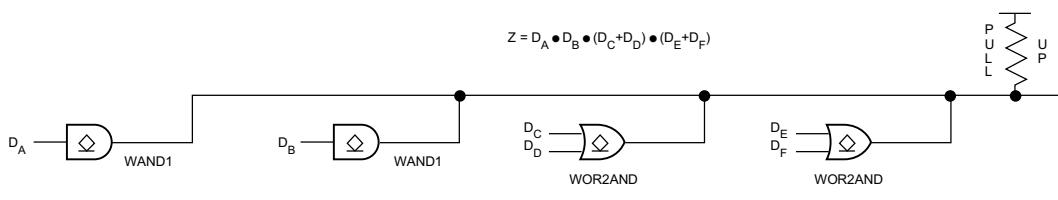
**Figure 21: Open-Drain Buffers Implement a Wired-AND Function**
