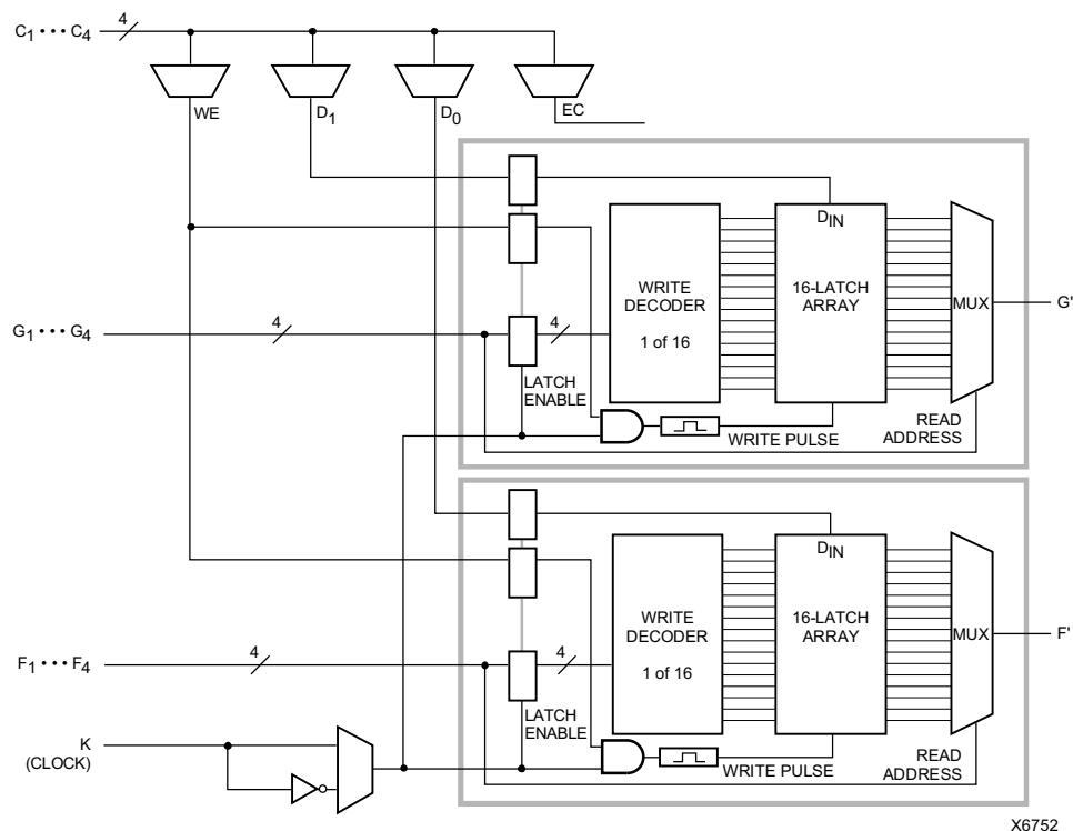
Figure 4: 16x2 (or 16x1) Edge-Triggered Single-Port RAM
