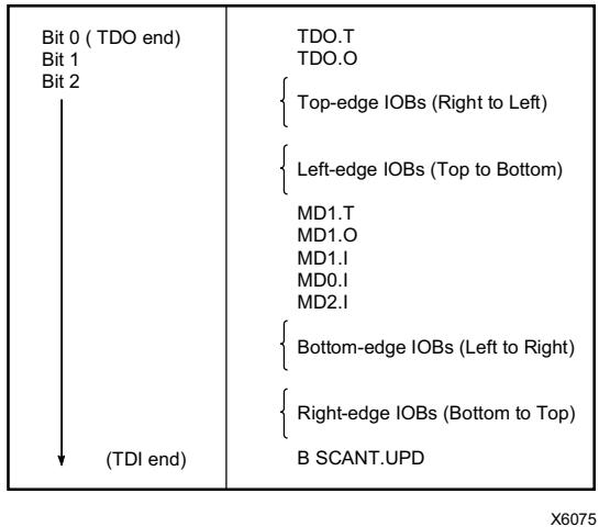
**Figure 42: Boundary Scan Bit Sequence**
