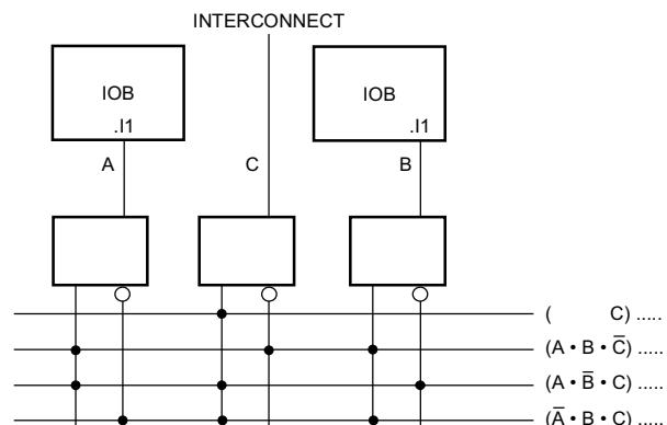
Figure 23: XC4000 Series Edge Decoding Example
