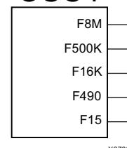
Figure 24: XC4000 Series Oscillator Symbol
