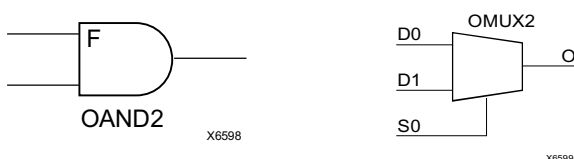
Figure 20: AND & MUX Symbols in XC4000X IOB
