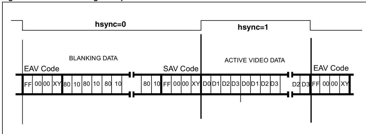
If manual mode is selected then the pixel positions for HSYNC rising edge and falling edge are programmable. The pixel position for the rising edge of HSYNC is programmed in the bHSyncRising registers. The pixel position for the falling edge of HSYNC is programmed in the bHSyncFalling registers.
