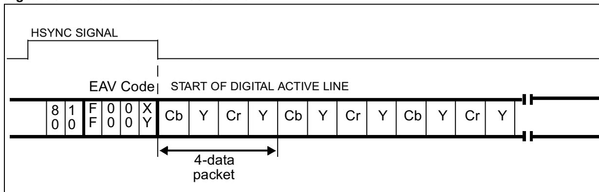
The VS6624 bYuvSetup register can be programmed to change the order of the components as follows:
