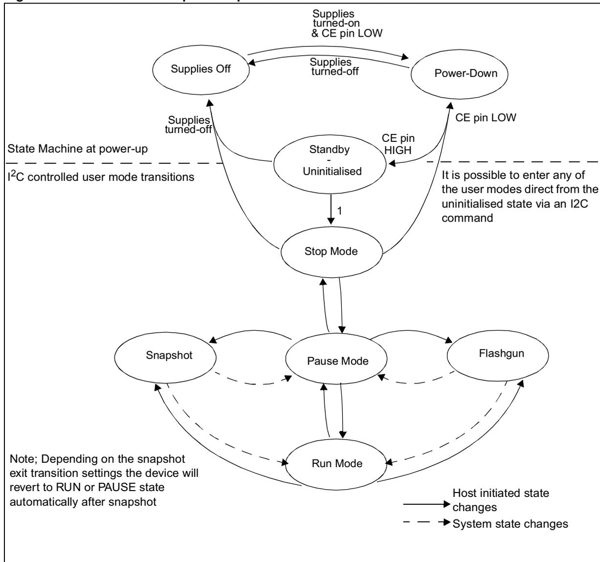
**Power Down/Up** The power down state is entered from all other modes when CE is pulled low or the supplies are removed. During the power-down state (CE = logic 0)
