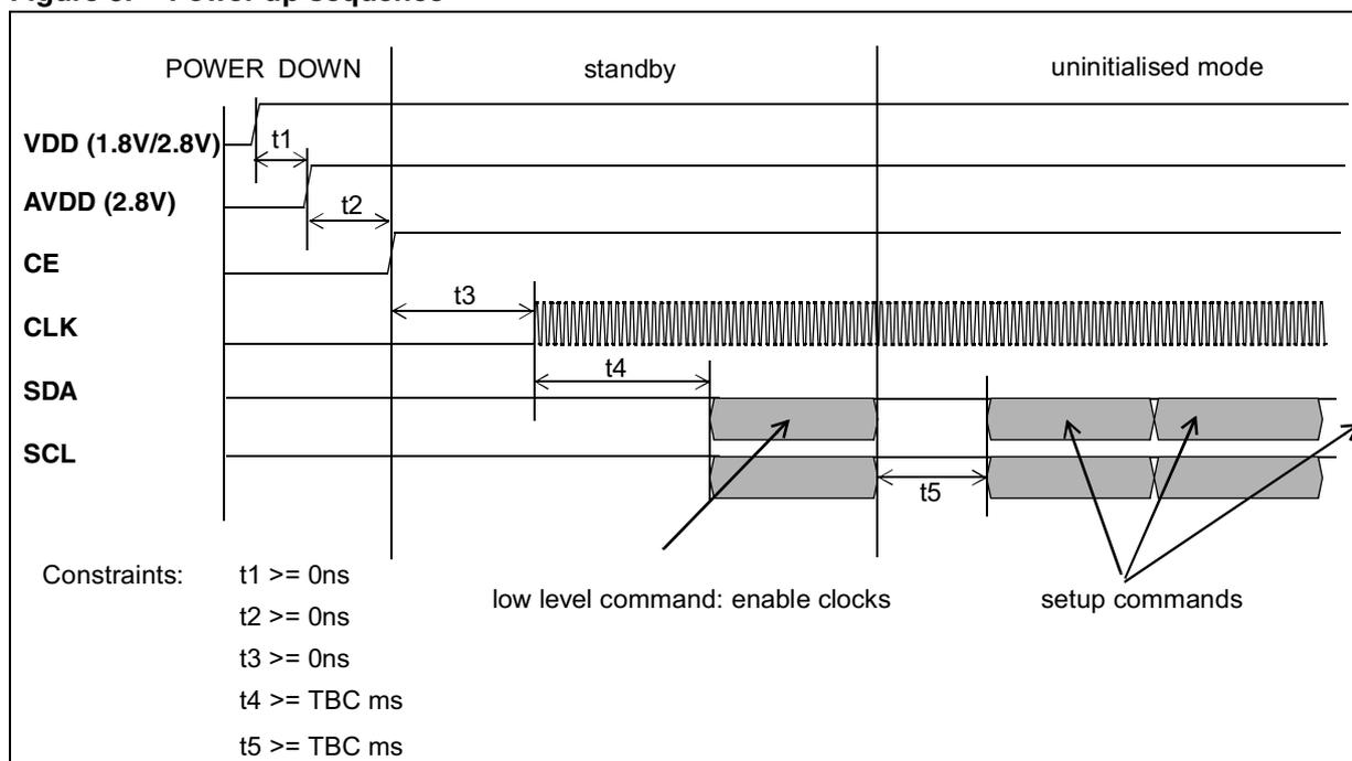
**STANDBY mode** The VS6624 enters STANDBY mode when the CE pin on the device is pulled HIGH. Power consumption is very low, most clocks inside the device are switched off.
