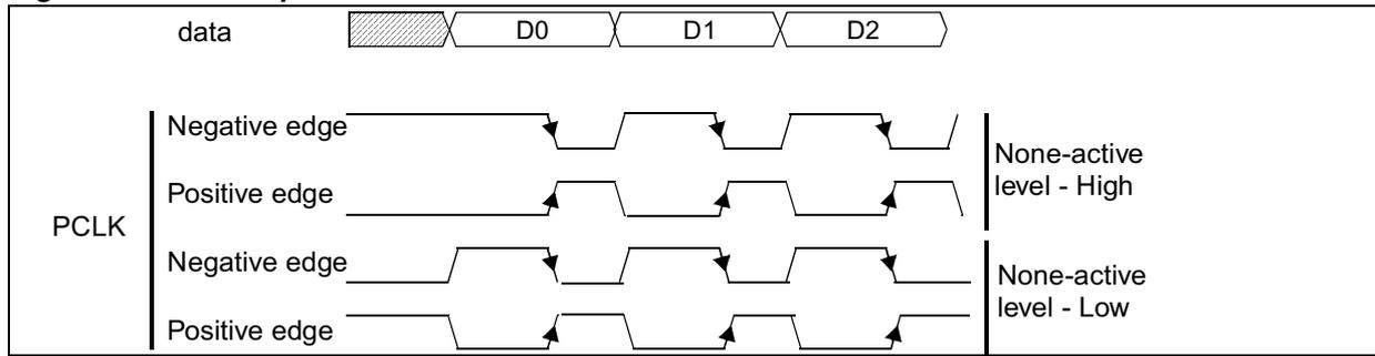
The YUV, RGB and bayer timings are represented on *Figure 17*, with the associated qualifying pclk clock. The output clock rate is effectively halved for the bayer 8-bit and YUV4:0:0 modes where only one byte of output data is required per pixel.
