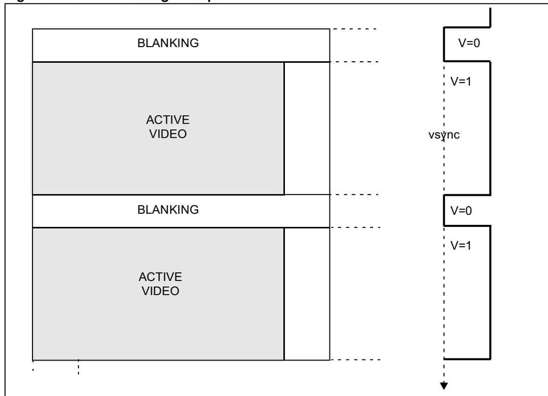
If manual mode is selected then the line number for VSYNC rising edge and falling edge is programmable. The rising edge of VSYNC is programmed in the bVsyncRisingLine registers, the pixel position for VSYNC rising edge is programmed in the bVsyncRisingPixel registers. Similarly the line count for the falling edge position is specified in the bVsyncFallingLine registers, and the pixel count is specified in the bVsyncFallingPixel registers.
