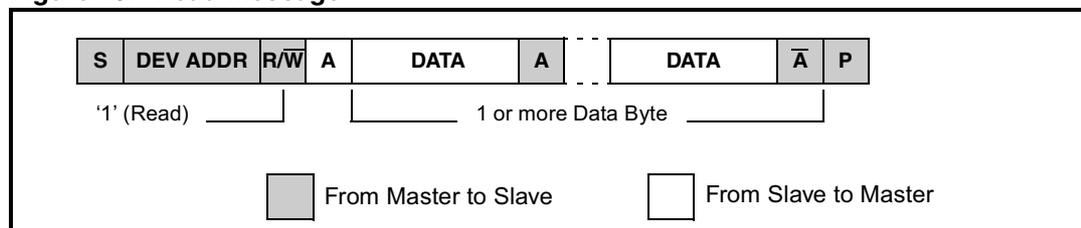
For the master reading from the slave the device address is followed by the contents of last register index that the previous read or write message accessed. If multiple data bytes are read then the internal register index is automatically incremented after each byte of data
