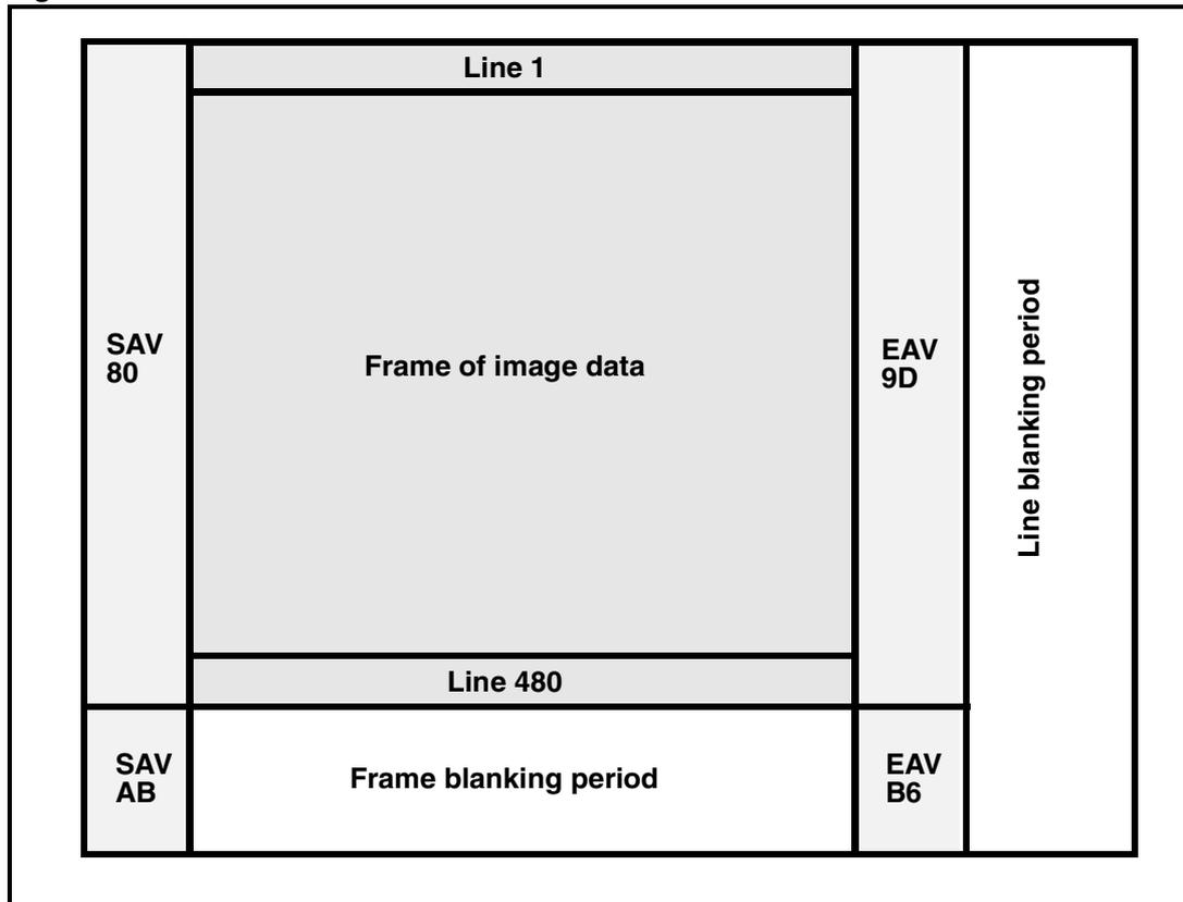
The synchronization codes for odd and even frames are listed in *Table 3* and *Table 4*. By default all frames output from the VS6624 are EVEN. It is possible to set all frames to be ODD or to alternate between ODD and EVEN using the SyncCodeSetup register in the *Output formatter control* register bank.
