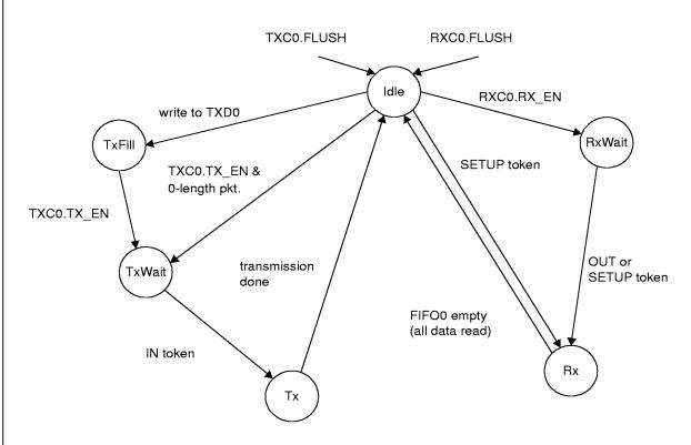
Figure 16. Endpoint 0 Operation
