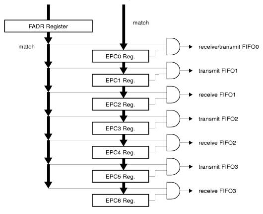
Figure 15. USB Function Address/Endpoint Decoding
