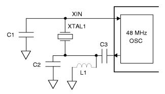
Figure 2. 3rd Harmonic Crystal Oscillator Connections
