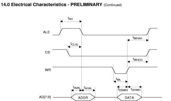
Figure 25. Multiplexed Mode Interface Write Timing
