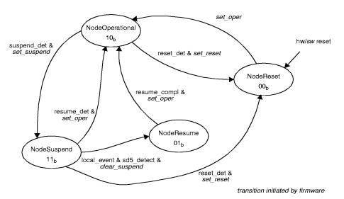
Figure 14. Node Functional State Diagram
