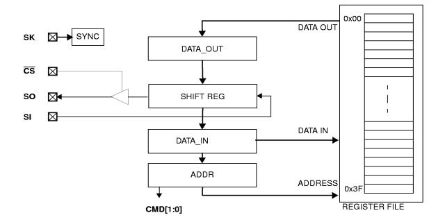
Figure 10. MICROWIRE Interface Block Diagram
