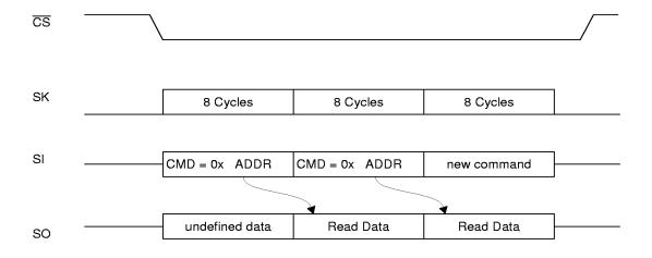
Figure 11. MICROWIRE Interface Basic Read Timing
