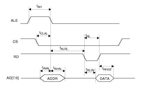
Figure 24. Multiplexed Mode Interface Read Timing
