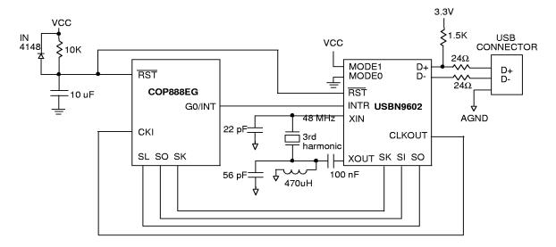
Figure 20. MICROWIRE Serial Interface
