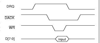
Figure 8. DMA Write to USBN9602
