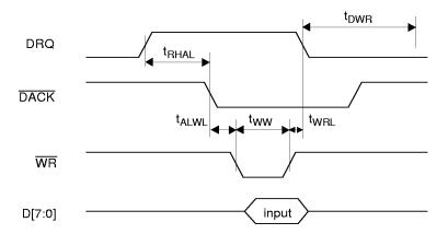
Figure 26. DMA Write to USBN9602
