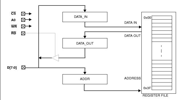
Figure 3. Non-Multiplexed Mode Interface Block Diagram
