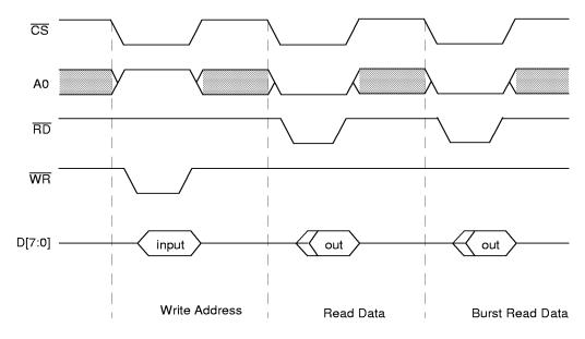
Figure 4. Non-Multiplexed Mode Basic Timing Diagram
