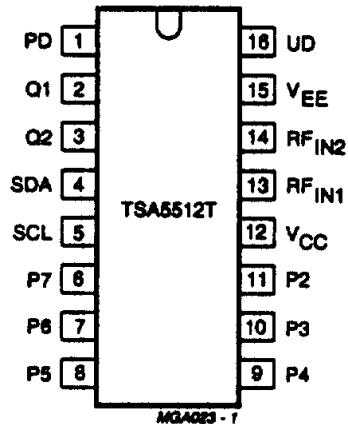
Fig.3 Pin configuration for SOT109.
