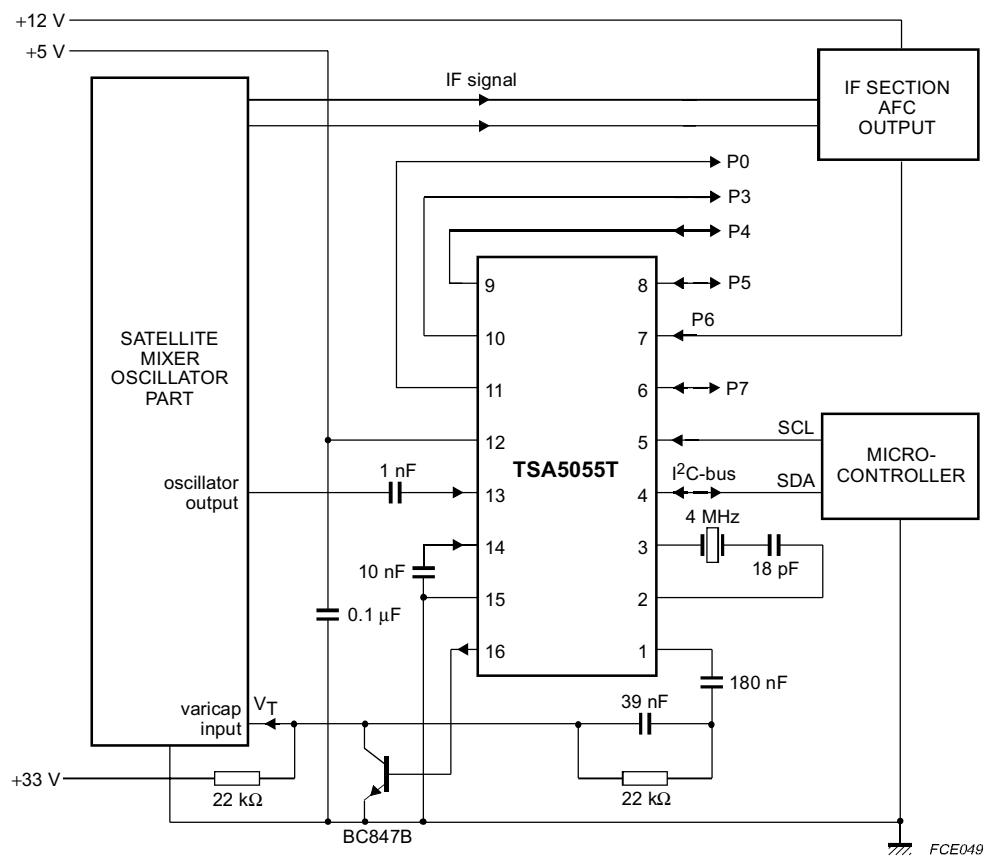
Fig.4 Asymmetrical application diagram.
