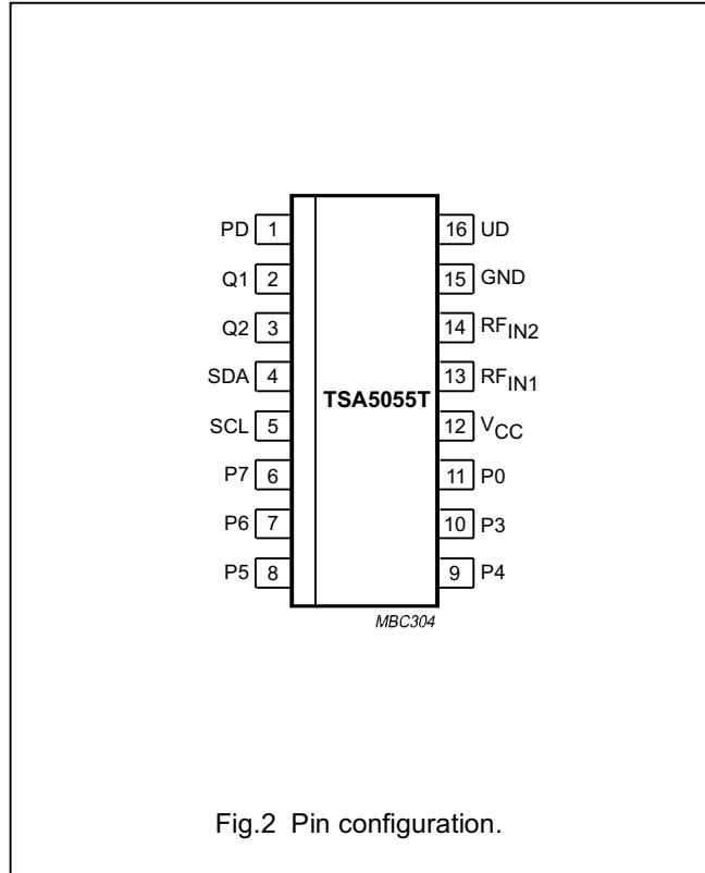
Fig.2 Pin configuration.
