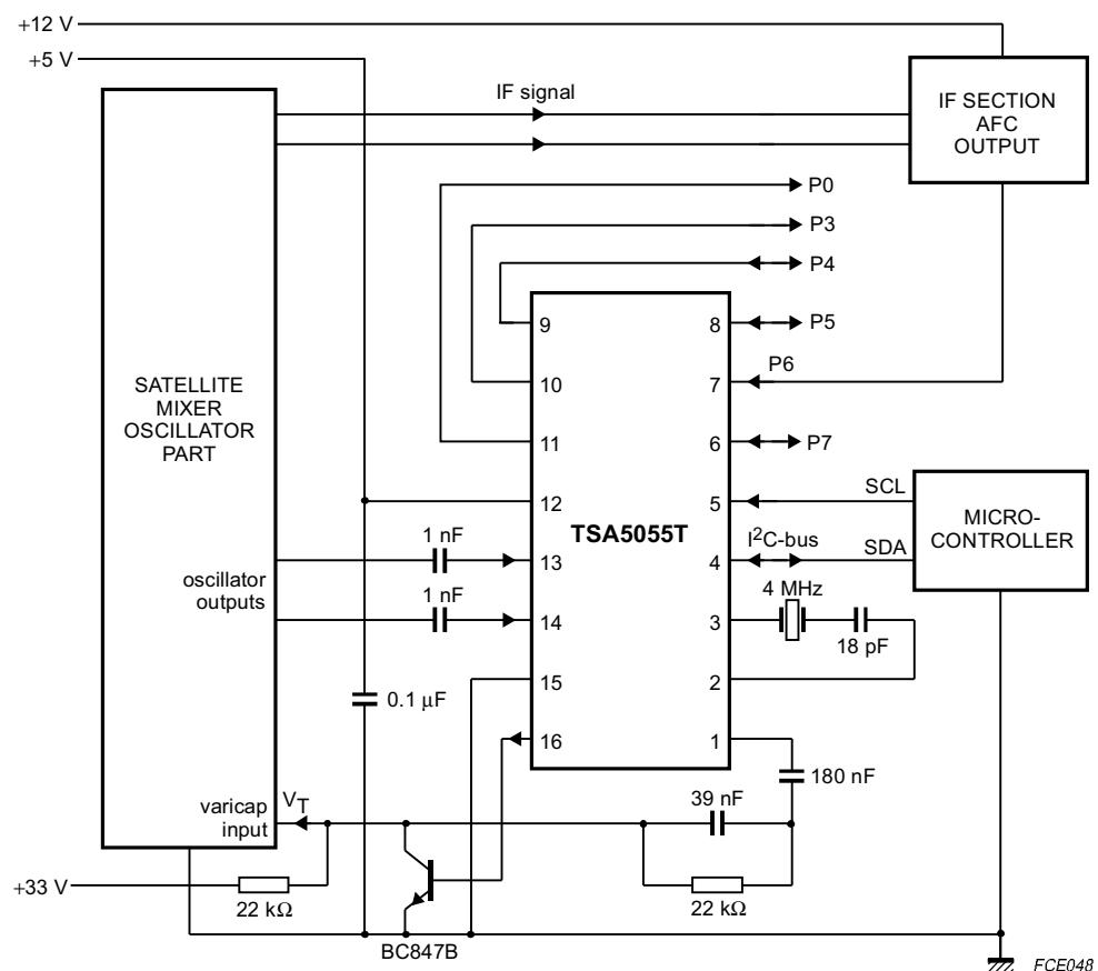
Fig.3 Symmetrical application diagram.
