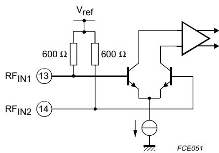
Fig.8 RF input amplifier.
