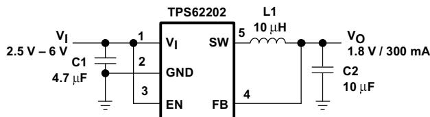
**Figure 1. Typical Application (Fixed Output Voltage Version)**
