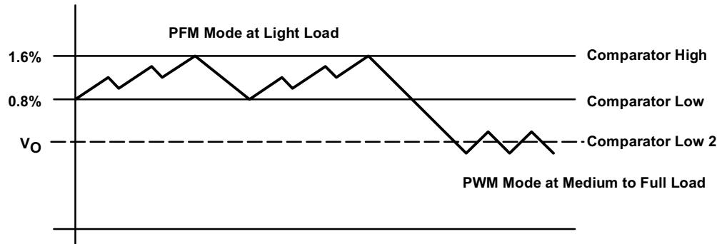
**Figure 2. Power Save Mode Thresholds and Dynamic Voltage Positioning**
