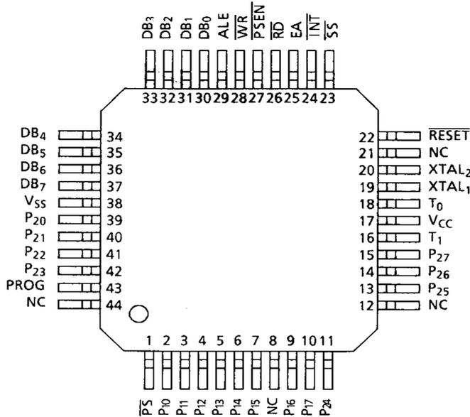
Figure 2.1 (2) Micro Flat Package Pin Connections
