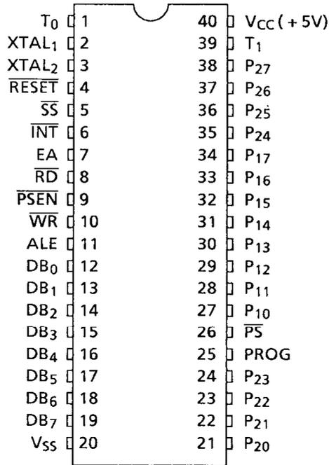
Figure 2.1 (1) DIP Pin Connections
