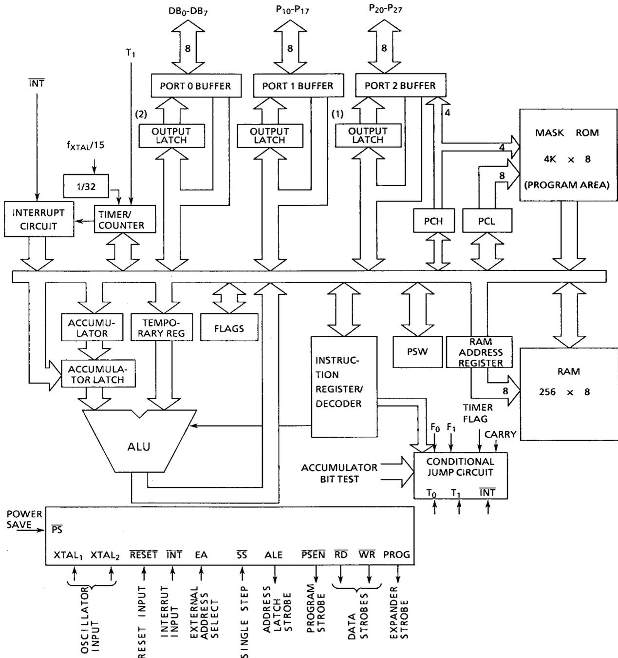
Note 1 : The lower order 4 bit of port 2 output latch are used also for input/output operations with the I/O expander.
