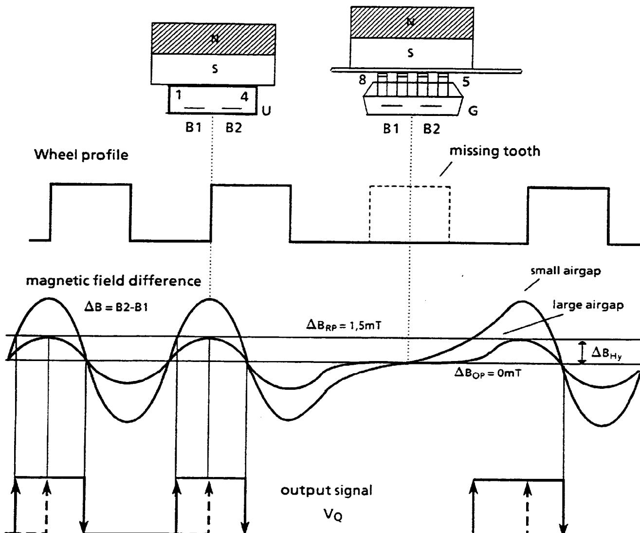
operate point:  $B_2 - B_1 < \Delta B_{OP}$  switches the output ON ( $V_Q = \text{LOW}$ )
