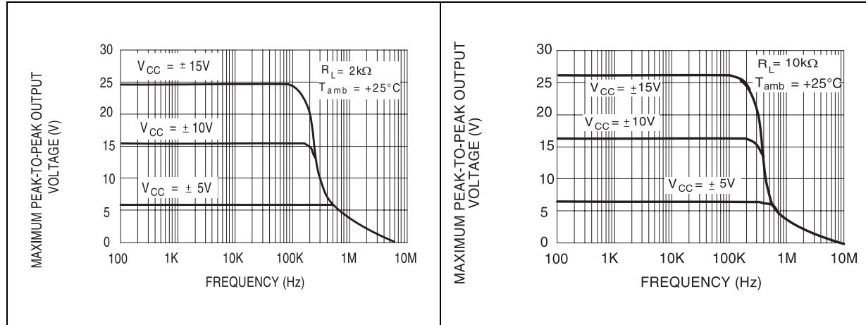
**Figure 4. Maximum peak-to-peak output voltage versus frequency**
