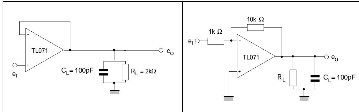
**Figure 20. Gain-of-10 inverting amplifier**
