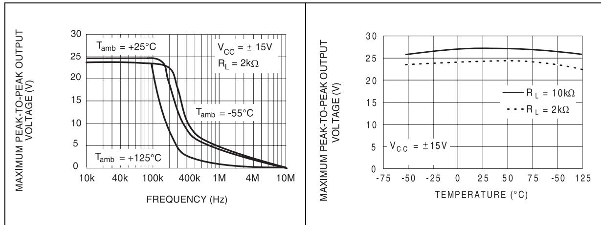
**Figure 6. Maximum peak-to-peak output voltage versus free air temp.**
