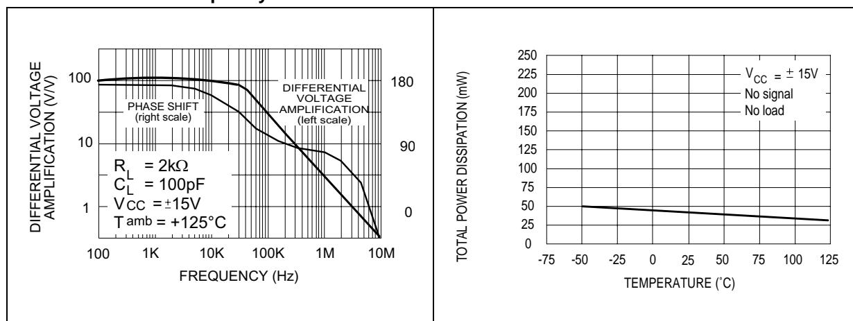
**Figure 12. Total power dissipation versus free air temperature**
