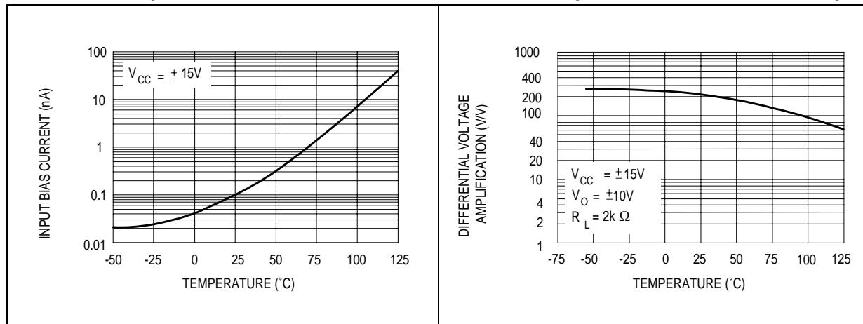
**Figure 10. Large signal differential voltage amplification versus free air temp.**
