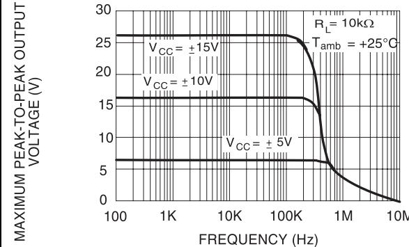
**Figure 5. Maximum peak-to-peak output voltage versus frequency**
