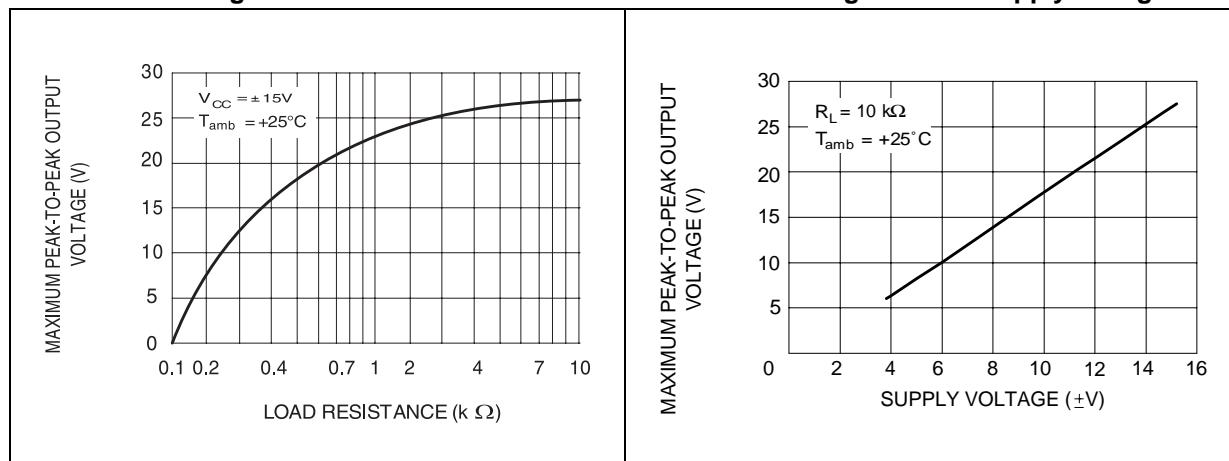
**Figure 8. Maximum peak-to-peak output voltage versus supply voltage**
