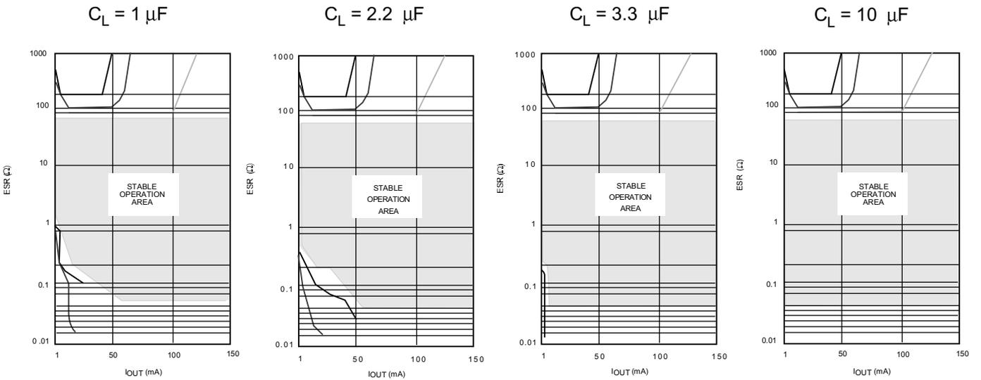
In general, the capacitor should be at least 1  $\mu\text{F}$  (aluminum electrolytic) and be rated for the actual ambient operating temperature range. The table below shows typical characteristics for several types and values of capacitance. Please note that the ESR varies widely depending upon manufacturer, type, size, and material.
