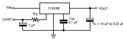
Note: Connect pin 5 to ground for heat sink
