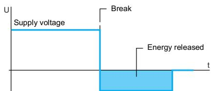
Coil voltage with diode protection module (--- only)
