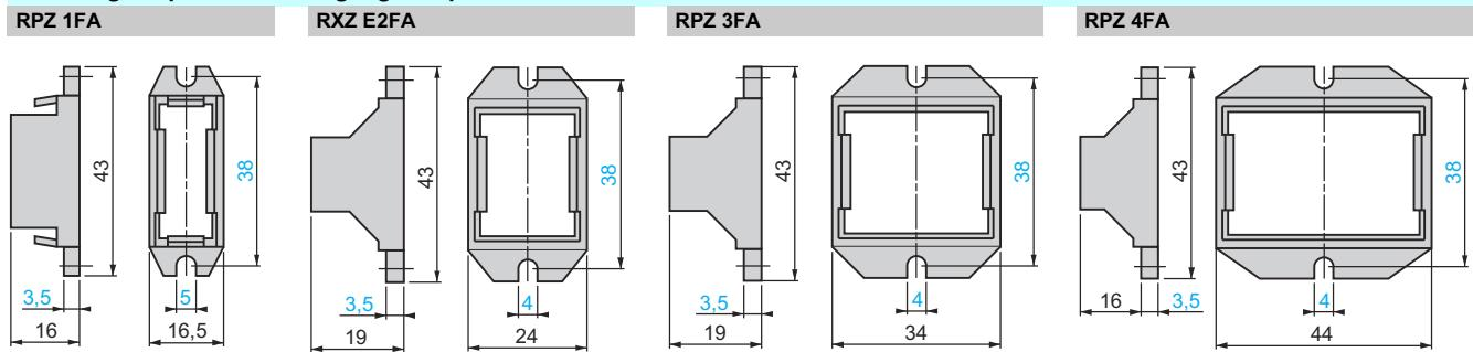
**Mounting**Mounting adapters for  $\text{U}_{\text{L}}$  rail (1)
