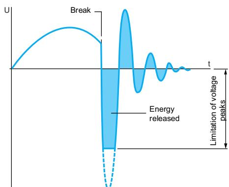
Coil voltage with varistor protection module (~/~ and ---)
