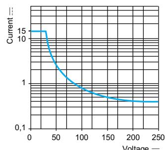
Durability (inductive load) = durability (resistive load) x reduction coefficient.
