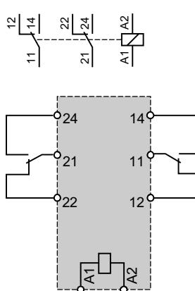
When using relay RSB 1A160●● with socket
