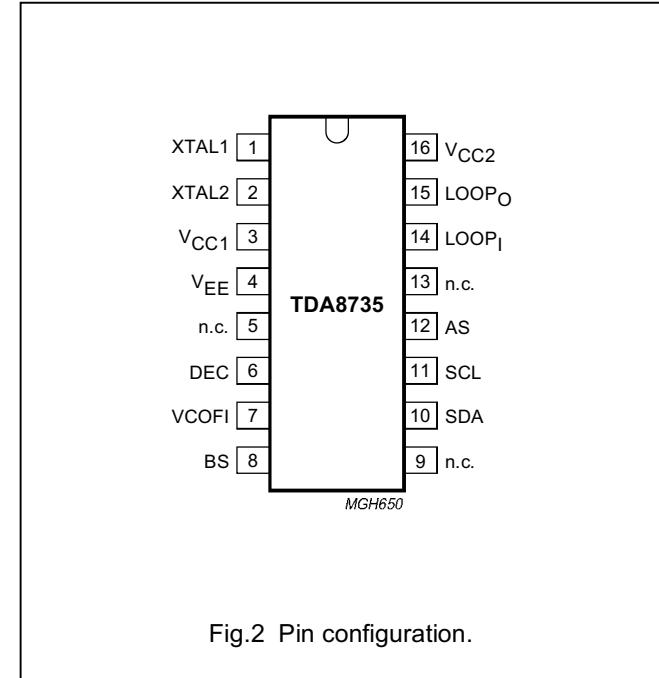
Fig.2 Pin configuration.
