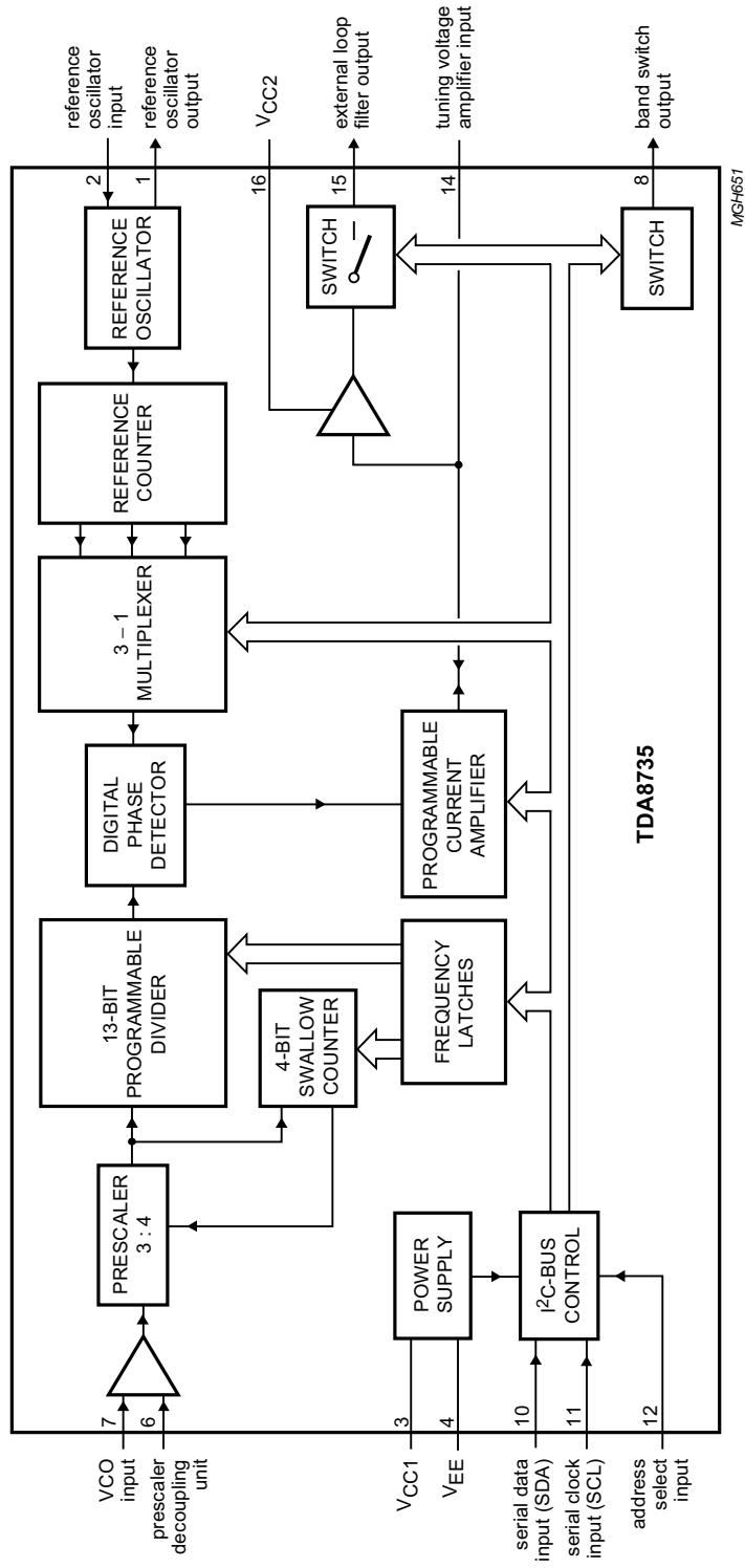
Fig.1 Block diagram.
