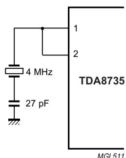
Fig.5 Crystal connection (4 MHz).
