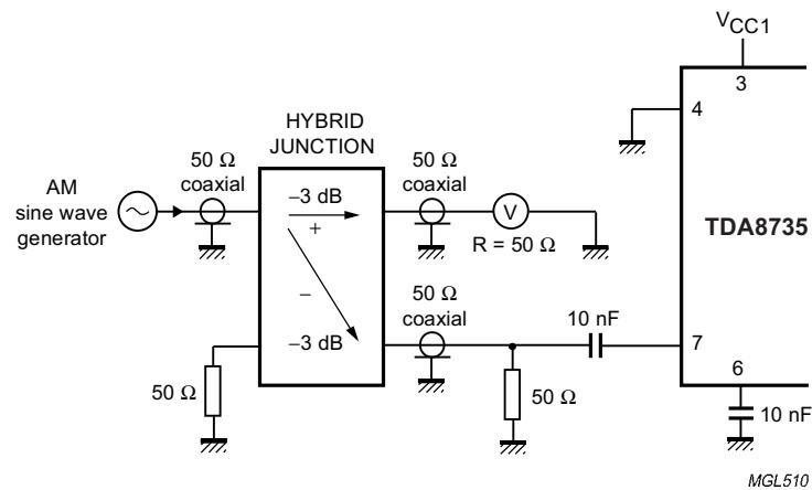
Fig.4 Prescaler input sensitivity (set-up measurement).
