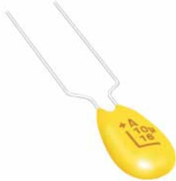
TAP is a professional grade device manufactured with a flame retardant coating and featuring low leakage current and impedance, very small physical sizes and exceptional temperature stability. It is designed and conditioned to operate to +125°C (see page 25 for voltage derating above 85°C) and is available loose or taped and reeled for auto insertion. The 15 case sizes with wide capacitance and working voltage ranges means the TAP can accommodate almost any application.
