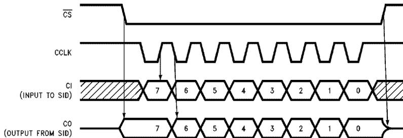
FIGURE 6b. TP3420A Alternate MICROWIRE Clock Format
