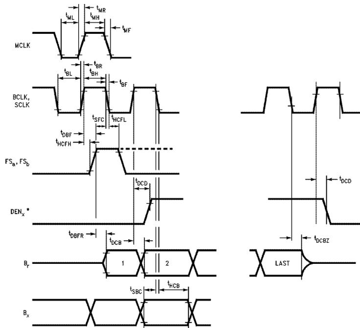
FIGURE 7. Timing Details for Digital System Interface
