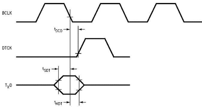
**FIGURE 9. Timing Details for TEM, DCKE Mode**
