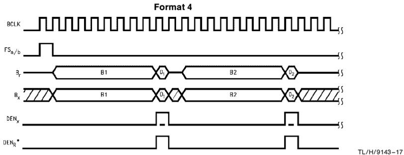
**FIGURE 3b. Digital System Interface Formats in TEM mode (DSI Master)**
