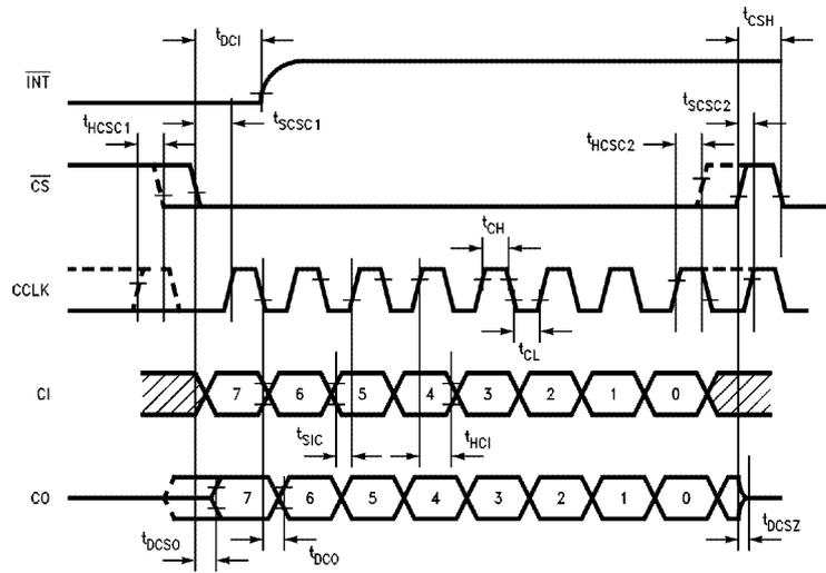
**FIGURE 4. TP3240A Enhanced MICROWIRE Control Interface Timing**
