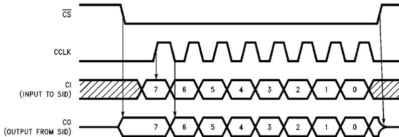
FIGURE 6a. TP3420A Normal MICROWIRE Clock Format
