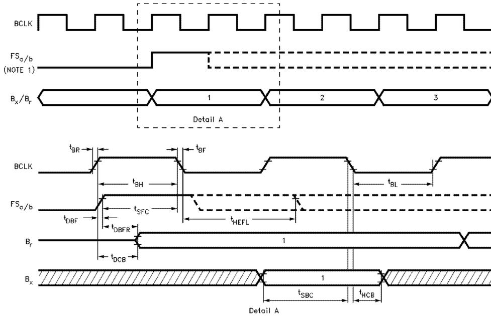
**FIGURE 8. Timing Details for Digital System Interface**
