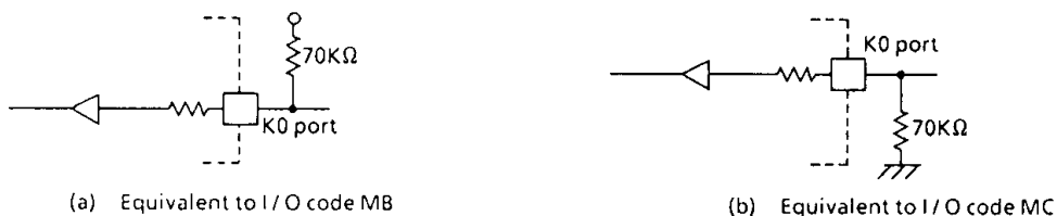
Figure 1-2. I/O code and external circuitry
