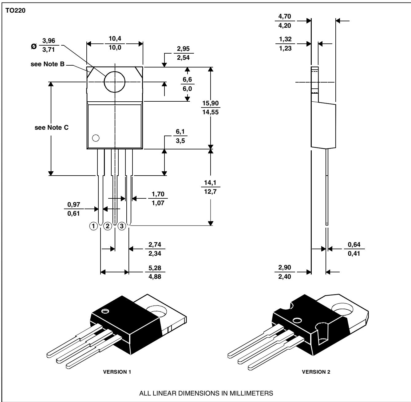
NOTES: A. The centre pin is in electrical contact with the mounting tab.
