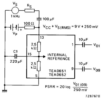
Fig. 14 Test circuit for PSRR for TEA0651/TEA0652.
