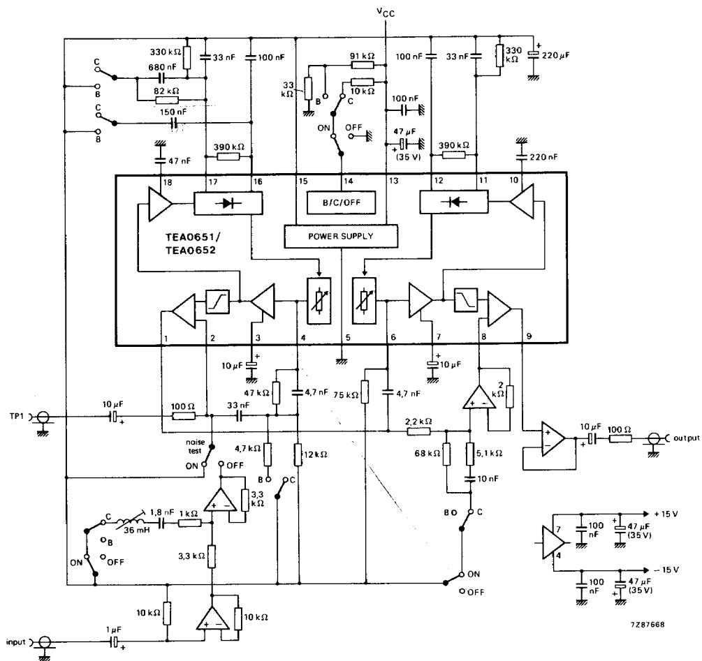
Fig. 13 Test circuit for TEA0651/0652. Encode mode.
