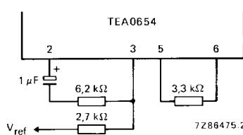
Fig. 21 Modification of Fig. 20 for  $V_{CC} \leq 11.5$  V.
