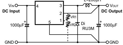
Use VR1 and VR2 only when adjusting the output voltages.
