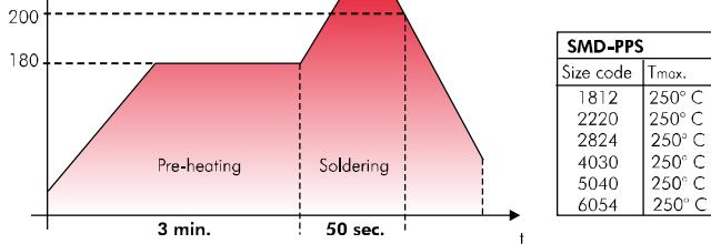
Temperature/time graph for the permissible processing temperature of the WIMA SMD film capacitor for typical convection soldering processes.
