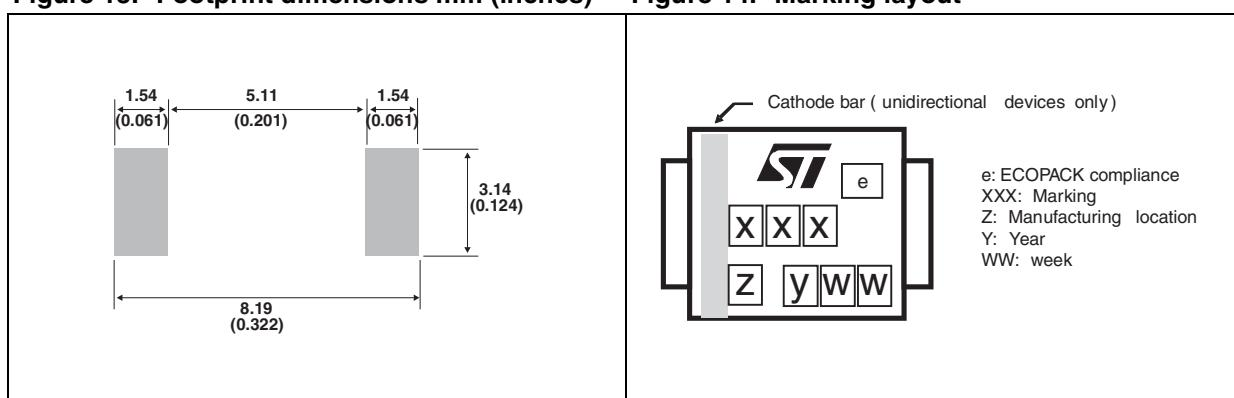
1. Marking layout can vary according to assembly location.
