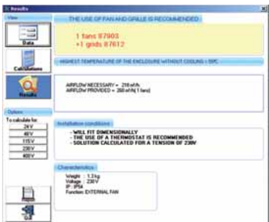
Select the thermal management system (fans, exchangers, etc.)
