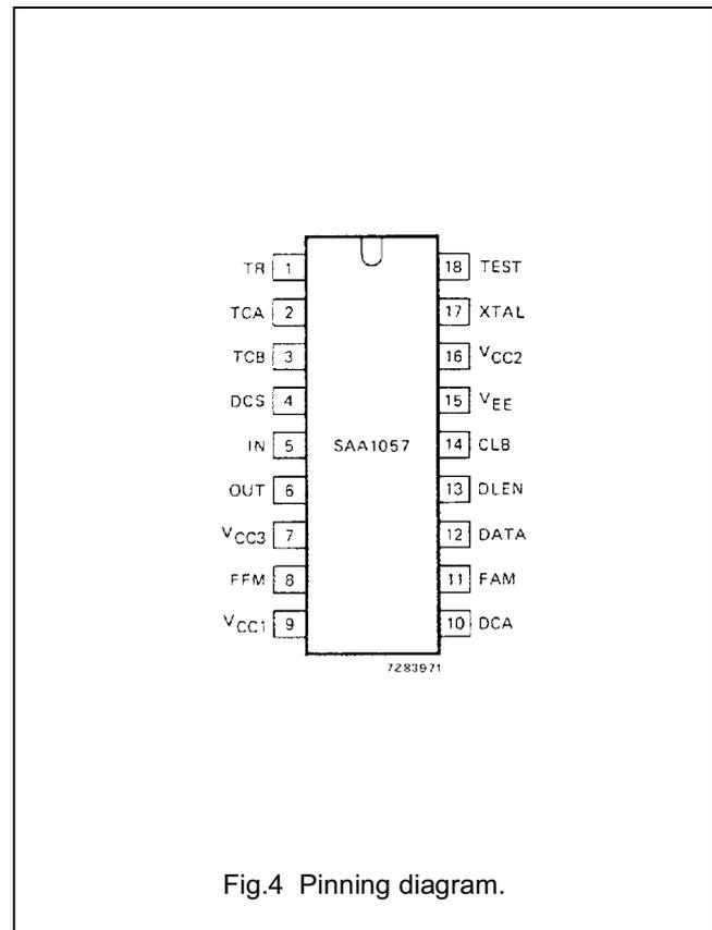
Fig.4 Pinning diagram.
