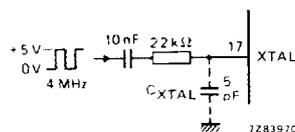
Fig.5 Circuit configuration showing external 4 MHz clock.
