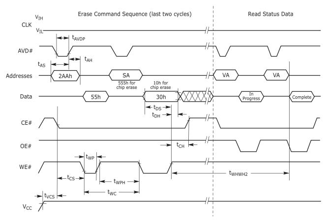
Figure II.14. Chip/Sector Erase Operation Timings
