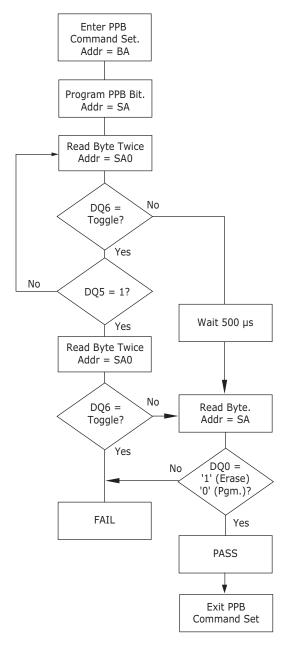
Figure 8.2. PPB Program/Erase Algorithm
