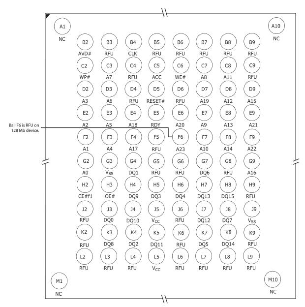
Figure 4.I. 84-ball Fine-Pitch Ball Grid Array (\$29W\$256N, \$29W\$128N)
