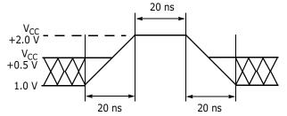
Figure II.I. Maximum Negative Overshoot Waveform
