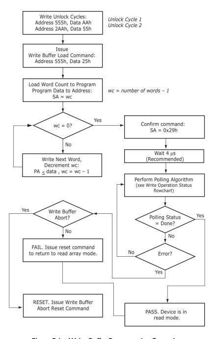
Figure 7.4. Write Buffer Programming Operation
