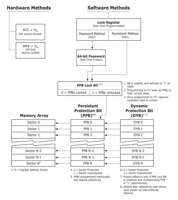
Figure 8.I. Advanced Sector Protection/Unprotection
