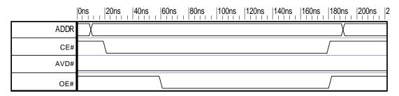
**Note:** DO2 polling during erase suspend behaves normally if CE# pulses low at or after valid Address, even if AVD# does not.
