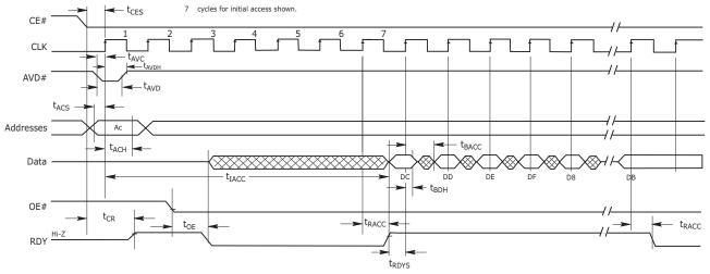
Figure II.8. 8-word Linear Burst with Wrap Around
