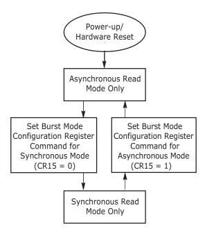
Figure 7.I. Synchronous/Asynchronous State Diagram
