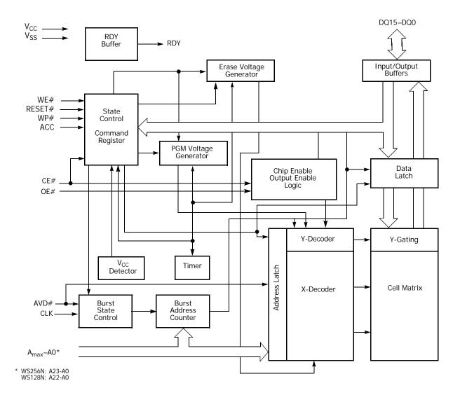
Figure 3.I. S29WS-N Block Diagram
