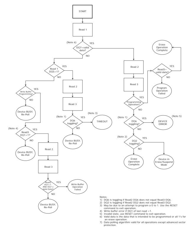
Figure 7.6. Write Operation Status Flowchart
