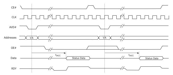
Figure II.19. Toggle Bit Timings (During Embedded Algorithm)
