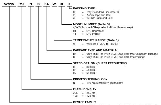
S29WS = 1.8 Volt-only Simultaneous Read/Write, Burst Mode Flash Memory
