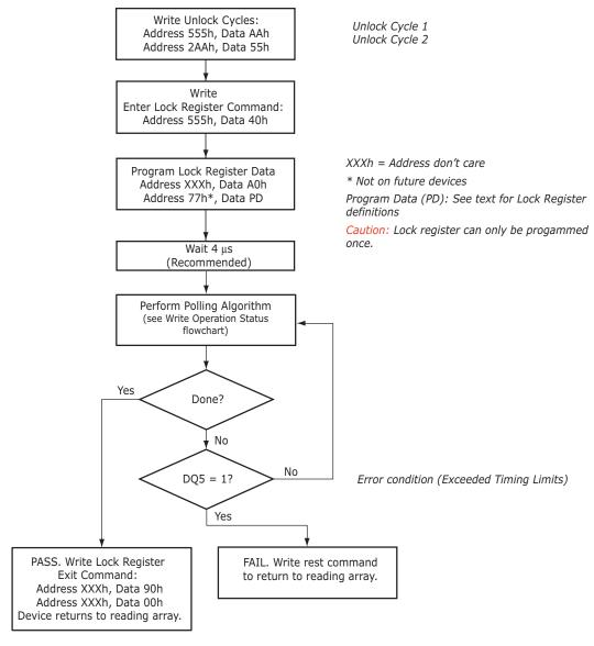
Figure 8.3. Lock Register Program Algorithm
