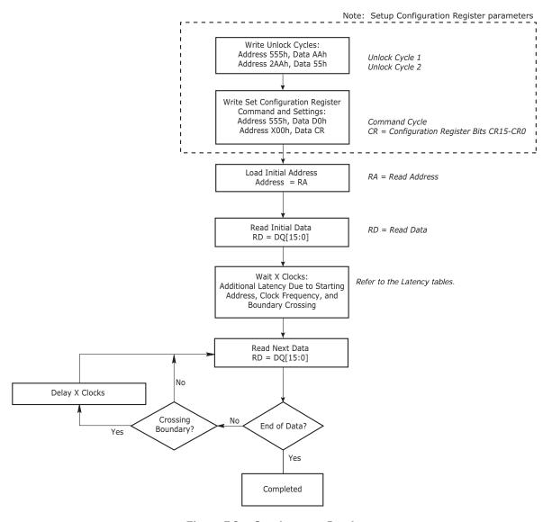
Figure 7.2. Synchronous Read
