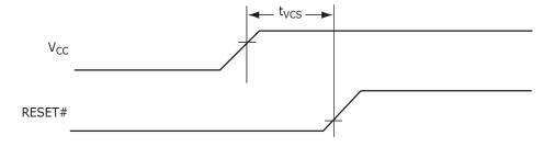
Figure II.5. V<sub>CC</sub> Power-up Diagram
