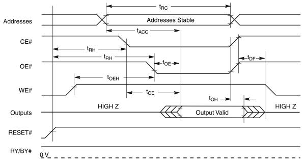
Figure I3. Read Operation Timings
