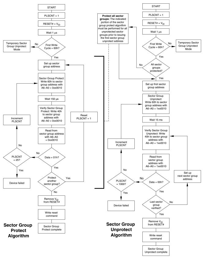
Figure 2. In-System Sector Group Protect/Unprotect Algorithms
