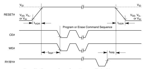
Figure 22. Temporary Sector Group Unprotect Timing Diagram
