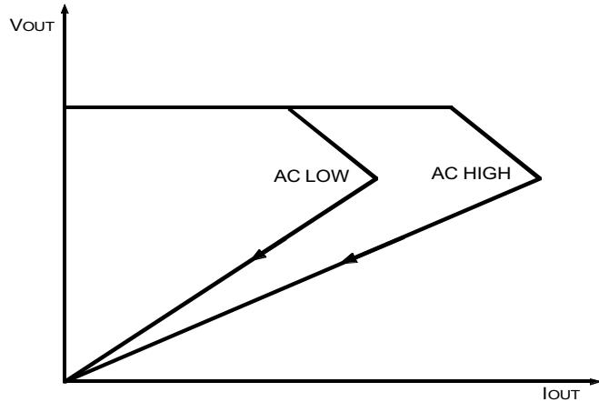
Figure 10 – Power Supply Output Overload Characteristics
