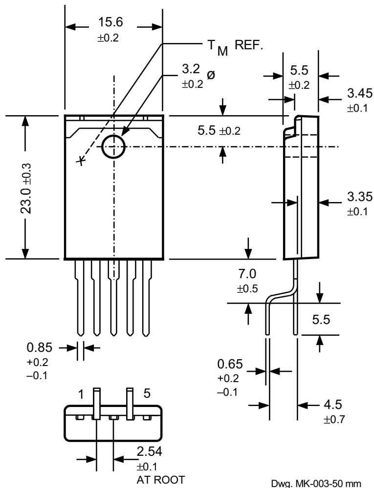
Recommended mounting hardware torque: 6 – 8 kg•cm or 0.588 – 0.784 Nm.
