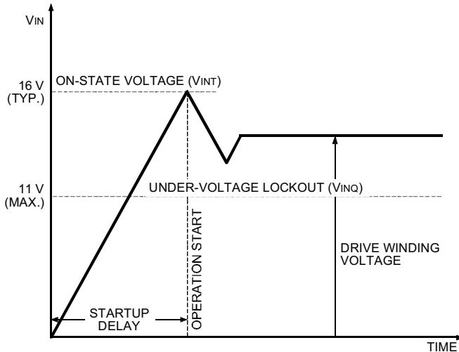
Figure 2 – Waveform of  $V_{IN}$  Terminal Voltage at Startup
