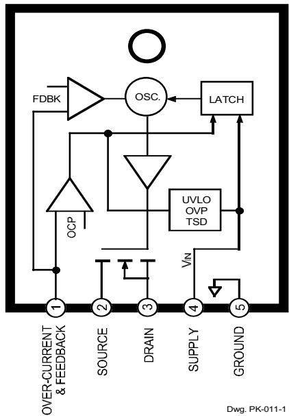
The Series STR-F6600 is specifically designed to satisfy the requirements for increased integration and reliability in off-line quasi-resonant flyback converters. The series incorporates a primary control and drive circuit with discrete avalanche-rated power MOSFETs.
