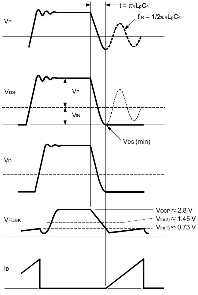
Figure 8 – Quasi-Resonance Waveforms
