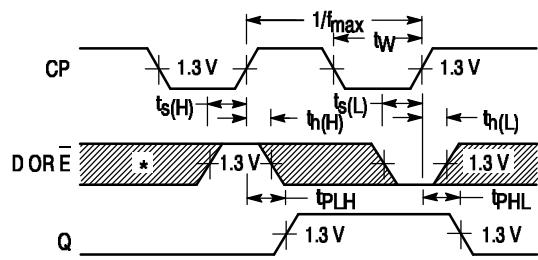
Figure 1. Clock to Output Delays Clock Pulse Width, Frequency, Setup and Hold Times Data or Enable to Clock
