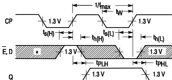
\*The shaded areas indicate when the input is permitted to change for predictable output performance.
