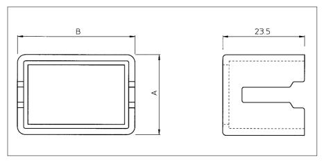
When pins are inserted into the panelmount receptacle half (SMS–R1) of the Quick mating connector, an optional pin protection shroud can be installed. The shroud is mounted at the same time as the receptacle by holding the shroud against the mating side of the panel with both cutouts lined up. The receptacle is then inserted in place, trapping the shroud between the receptacle and panel. The use of the pin protection shroud reduces the allowable thickness of the panel from 2.3 to 1.6 mm max.
