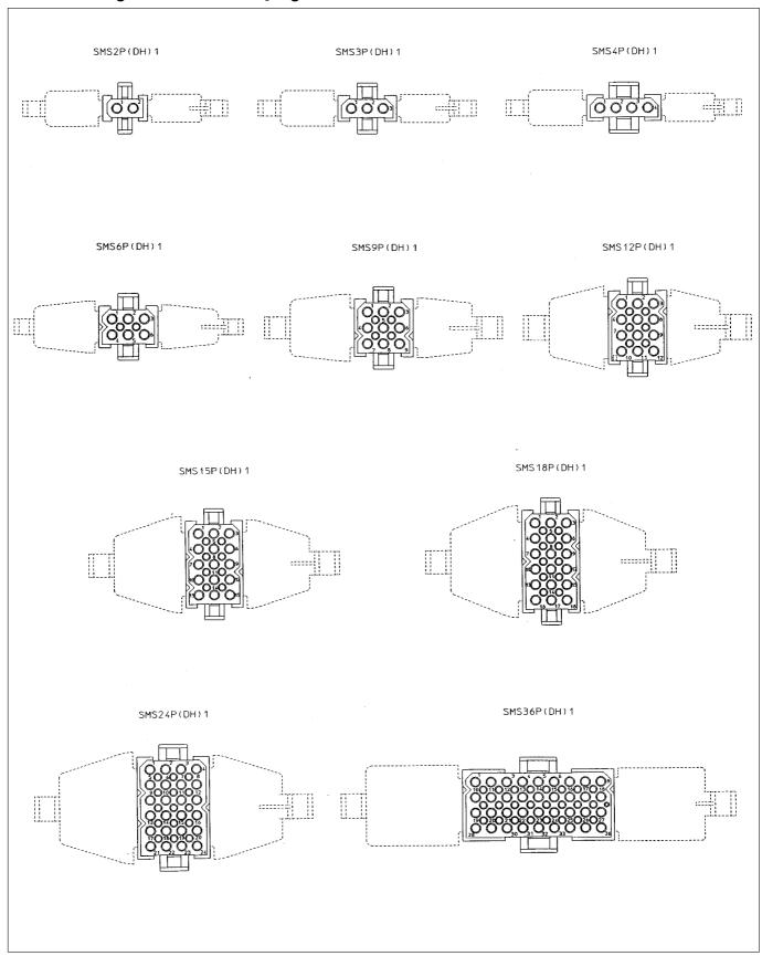
Contact identifications shown are for mating face. Contact identifications of wiring face are identical as shown on the receptacle arrangements
