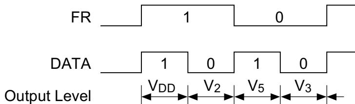
COM0– LCD common (row) driving output. One of the VDD, V1, V4 and V5 levels is selected by a combination of the output of the common counter and the FR (COM31– COM15) signal. The common (row) scanning order for the slave LSI is reverse to that for COM16) the master LSI.
