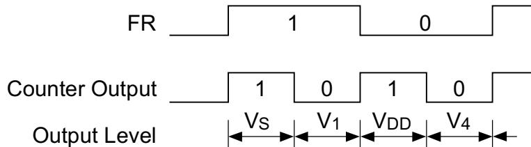
M/S Input signal which selects the master or slave LSI. Connected to VDD or Vss.
