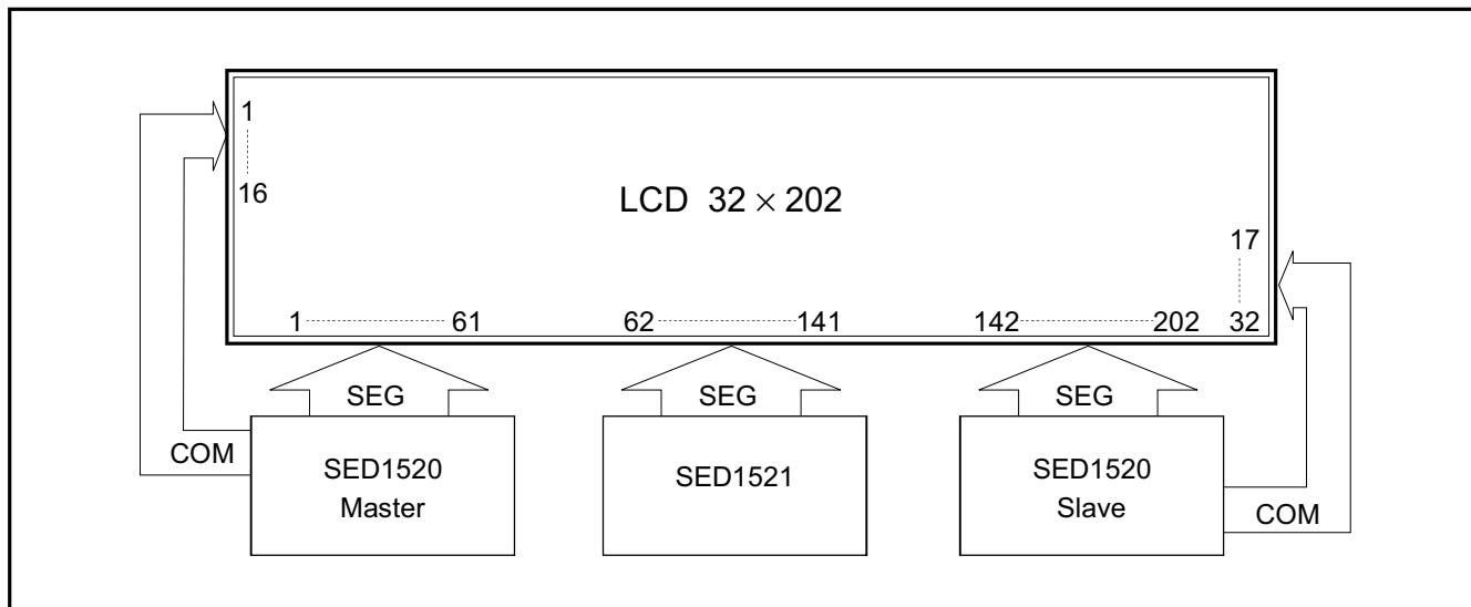
\* SED1521F may be omitted. If it is not used, the panel consists of 32 × 122 dots.
