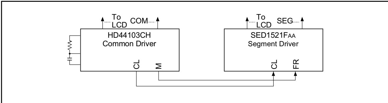
\*1. In this connection, the duty of the SED1521FOA must be the same as that of the SED1520FOA.
