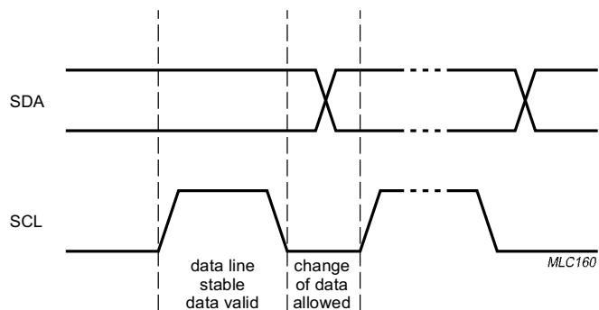
Fig.7 Bit transfer on the I<sup>2</sup>C-bus.
