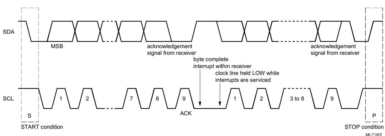
Fig.9 Data transfer on the I<sup>2</sup>C-bus.
