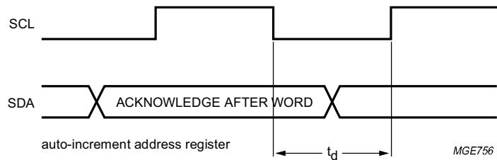
Fig.11 Timing of reduced I<sup>2</sup>C-bus frequency.
