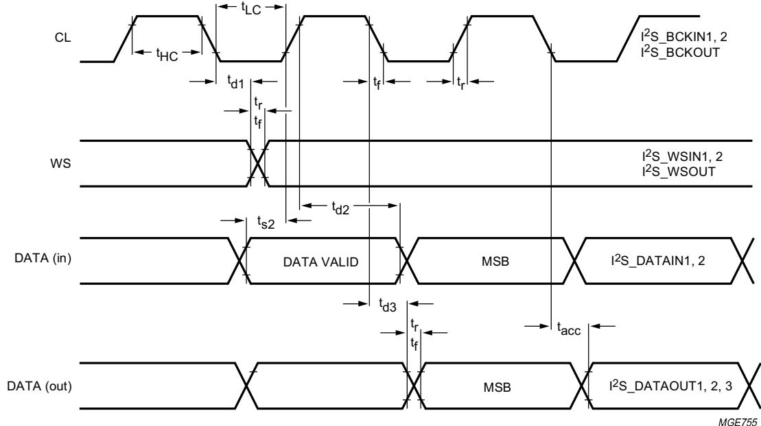
Fig.6 Timing diagram of I<sup>2</sup>S-bus output interface.
