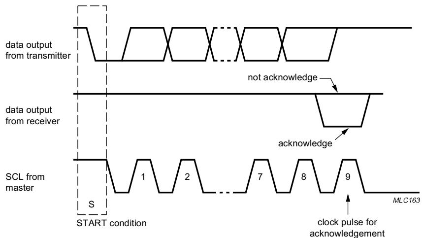
Fig.10 Acknowledge on the I<sup>2</sup>C-bus.
