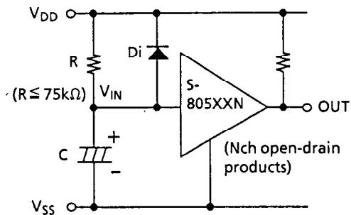
Note 1:  $R$  should be  $75\text{k}\Omega$  or less for purpose of protection against oscillation.
