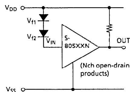
$$\text{Detection voltage} = V_{f1} + V_{f2} + -V_{DET}$$
