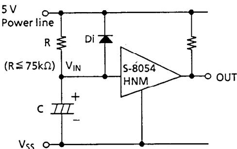
Note 1: R should be  $75\text{k}\Omega$  or less for purpose of protection against oscillation.
