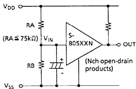
$$\text{Detection voltage} = \frac{RA + RB}{RB} \cdot -V_{DET}$$
