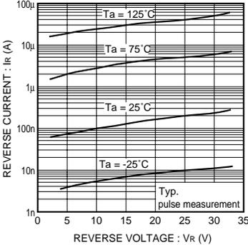
Fig. 2 Reverse characteristics
