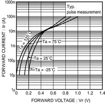
Fig. 1 Forward characteristics
