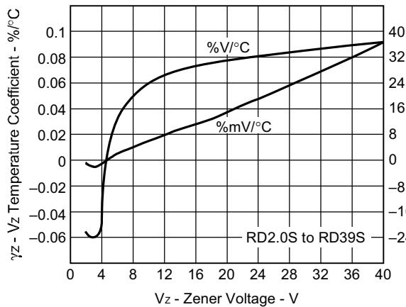
**Fig. 10 ZENER VOLTAGE TEMPERATURE COEFFICIENT vs. ZENER VOLTAGE**
