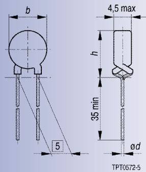
TPT0572-5                                       | V <sub>max</sub> = 20 V, T <sub>Ref</sub> = 150 °C  | C1165                                              | 800                                                  | 1<br>9,0    12,5    0,6          | Anwendung in Ladegeräten/Charger applications<br>bis/up to 15 V<br>B59165-C1150-A70                                                                                                                                              |
