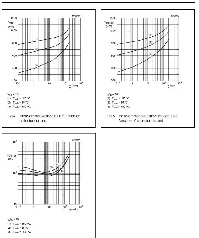
Fig.6 Collector-emitter saturation voltage as a function of collector current.
