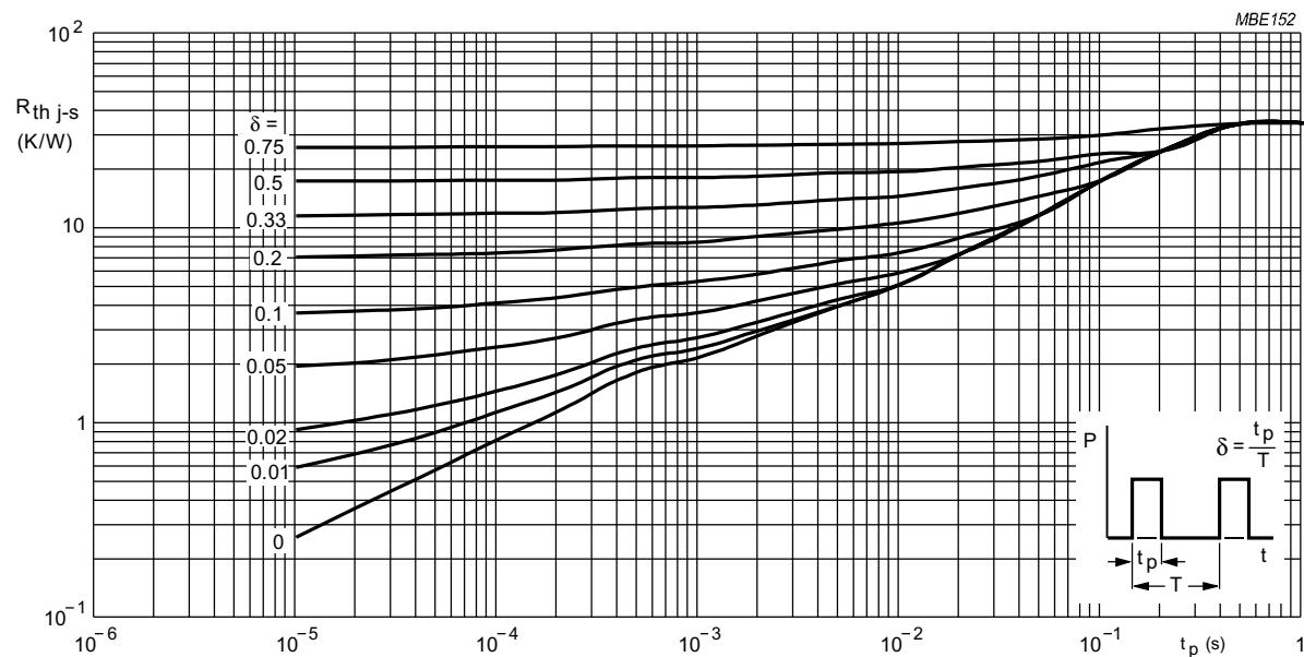
Fig.20 Transient thermal resistance from junction to soldering point as a function of pulse time; typical values.
