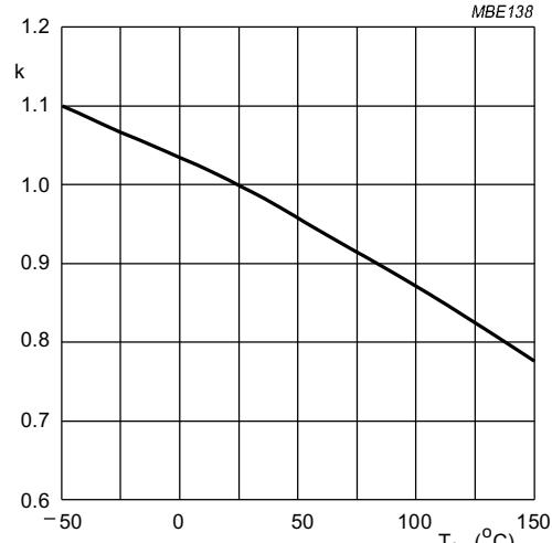
$$k = \frac{V_{GSth} \text{ at } T_j}{V_{GSth} \text{ at } 25^\circ\text{C}}$$
