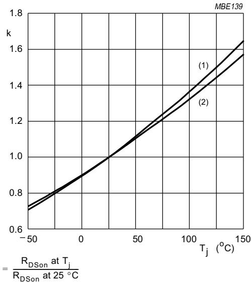
$k = \frac{R_{DSon} \text{ at } T_j}{R_{DSon} \text{ at } 25^\circ\text{C}}$
