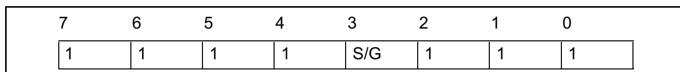
Figure 26 MONITOR Channel on IDP0
