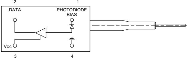
**Figure 1. P171-Type R-PAK PIN/Preamp Schematic (Top View)**
