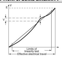
The independent linearity (conformity for the non linear laws) is the maximum gap  $\Delta V$  between the actual variation curve and the theorical variation curve the nearest to it. The linearity and the conformity are expressed in percentage of the total applied voltage E
