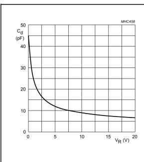
f = 1 MHz;  $T_{amb} = 25 \,^{\circ}\text{C}$ .
