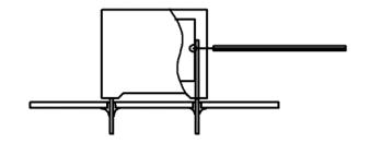
Temperature monitored inside the capacitor.
