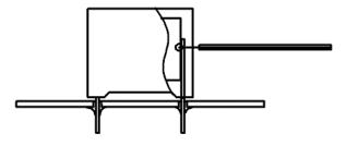
Temperature monitored inside the capacitor.
