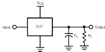
C<sub>L</sub> includes load and stray Capacitance
