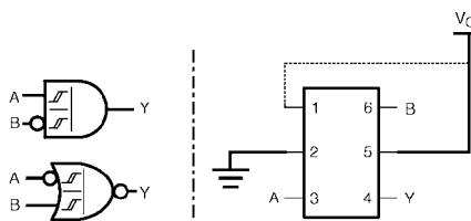
FIGURE 8. 2-Input AND with Inverted B Input
