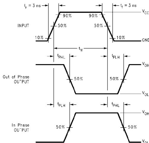
FIGURE 13. AC Waveforms
