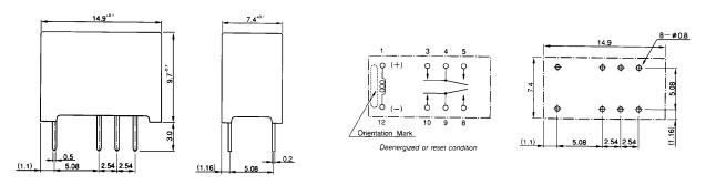
NAL-D type (double winding latching type)
