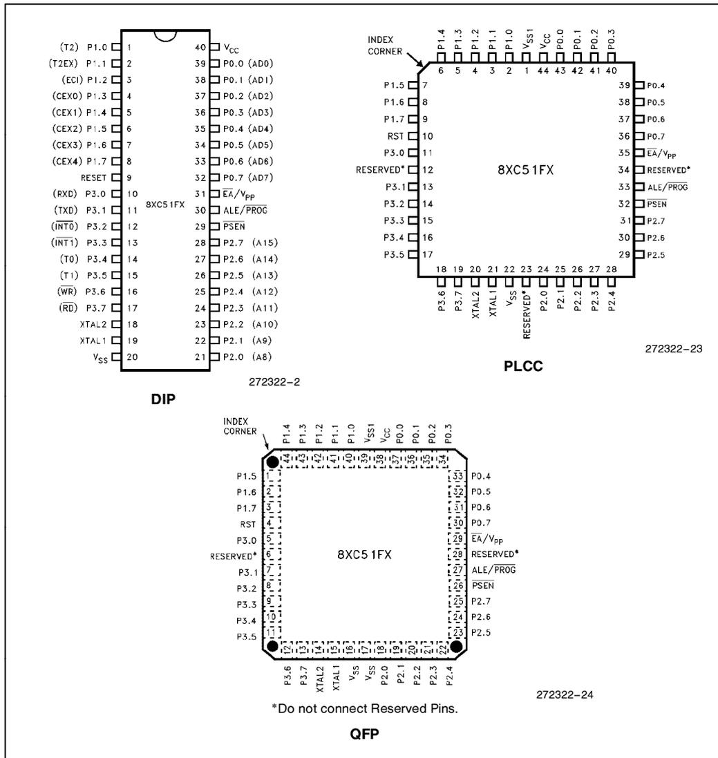
Figure 2. Pin Connections
