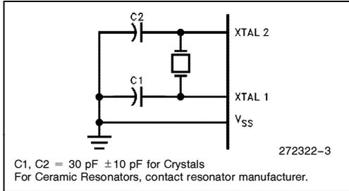
Figure 3. Oscillator Connections
