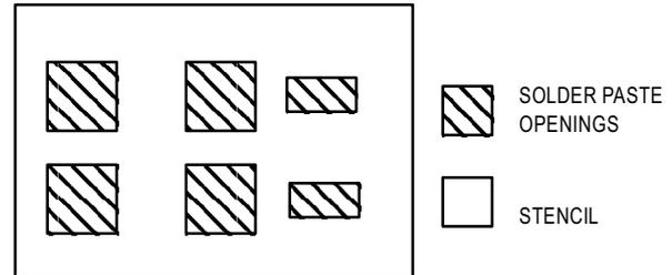
**Figure 16. Typical Stencil for DPAK and D<sup>2</sup>PAK Packages**
