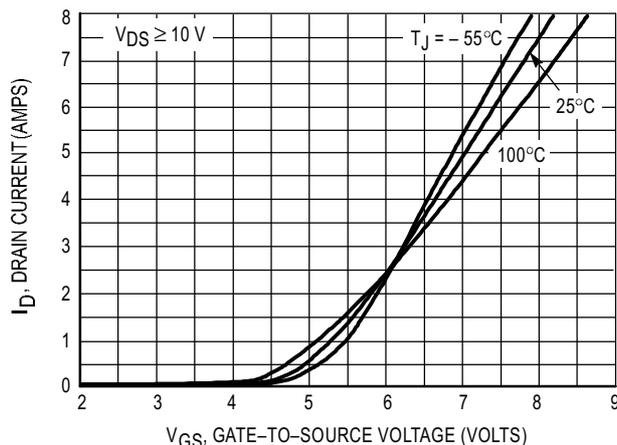
Figure 2. Transfer Characteristics
