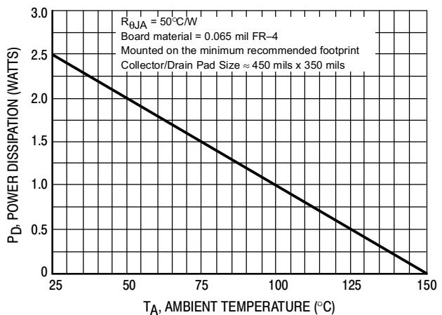
Figure 15. D<sup>2</sup>PAK Power Derating Curve
