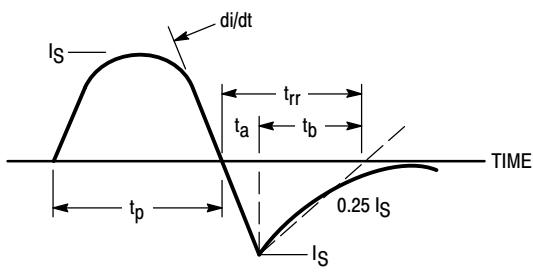
Figure 14. Diode Reverse Recovery Waveform
