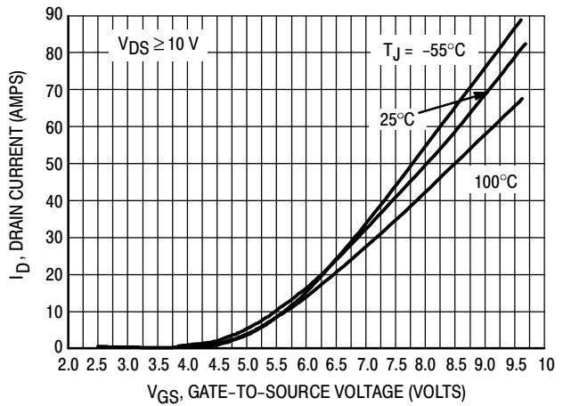
Figure 2. Transfer Characteristics
