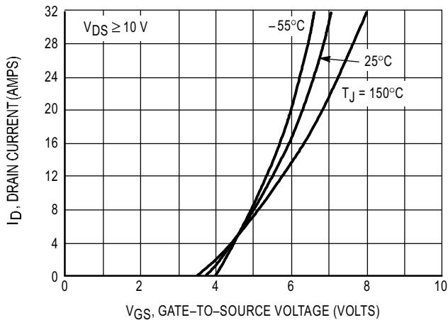
Figure 2. Transfer Characteristics
